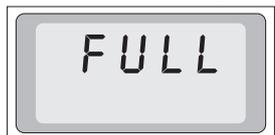
To store the current sample, press the STO button again and this will overwrite the oldest sample in the memory. All samples are shifted (reference numbers reduced by one). Sample number one remains the oldest sample.
