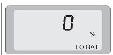
When the batteries are too weak to ensure reliable measurements, the message 0% LO BAT appears for a few seconds, and then the meter will automatically switch itself off. Replace the batteries immediately.
